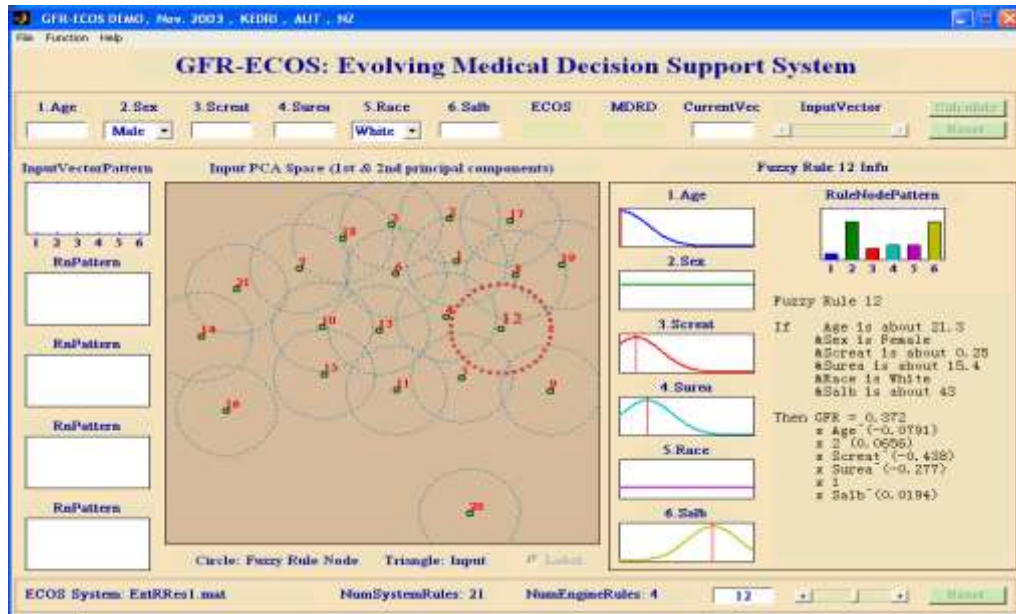
Figure 18. Example of a DENFIS application system using six input variables to train a DENFIS system for a medical decision support on a renal function GFR, where the evolved hidden nodes represent clusters of input data and the data in each of these clusters is approximated by a regression function ([37]).
