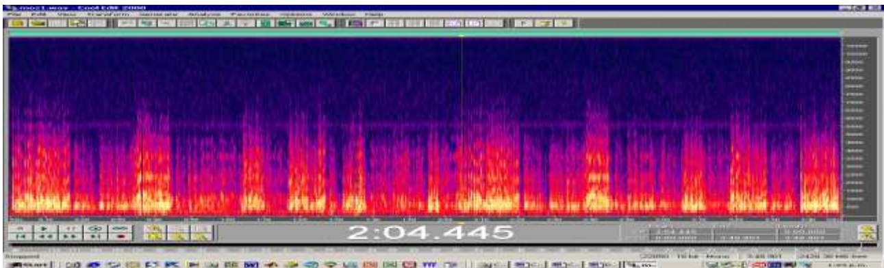
Figure 10. A spectrogram of the Mozart's music from fig.6, representing the power of frequencies (on the y axis) over time (on the x axis) as spectro-temporal data.
