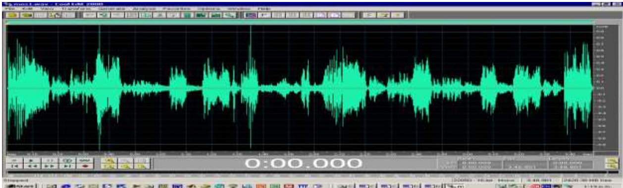
Figure. 6. A wave form of a segment from Mozart's music, represented as intensity of the sound over time, contains spectro-temporal information.
