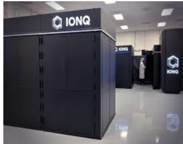
IonQ Quantum Computer Trapped ion device: 36 qubits
